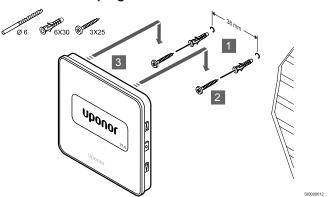
Attach the thermostat to the wall using the screw and wall plug.
