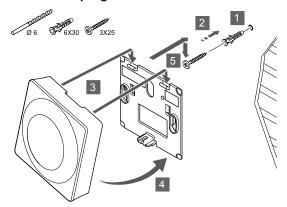
Attach the thermostat to the wall using the screw and wall plug.
