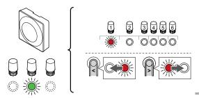
Use buttons < or > to move the pointer (LED flashes red) to a preferred channel.
