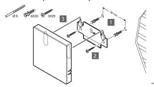
Attach the thermostat to the wall using the wall bracket, screws and wall plugs.
