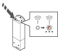
Press and hold the register button on the relay module until the LEDs on the module start flashing slowly.
