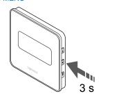
Press and hold the **OK** button for about 3 seconds to exit the settings menu.
