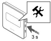
Press and hold the **OK** button for about 3 seconds. The settings icon and menu numbers is displayed in the top right corner of the display.
