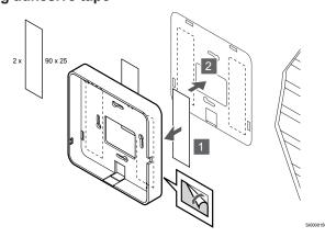
Attach the communication module back mount to the wall using adhesive tape.
