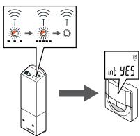
The connection indicator starts flashing in the thermostat display to show that the registration process begins.
