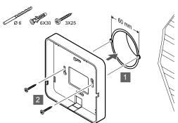
Attach the communication module back mount to the wall box.
