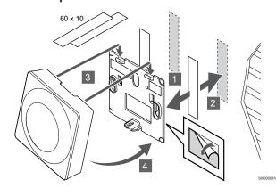
Attach the thermostat to the wall using the wall bracket and adhesive strips.
