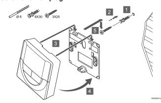
Attach the thermostat to the wall using the screw and wall plug.
