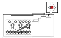
Use buttons < or > to move the pointer to the power LED (LED flashes red).
