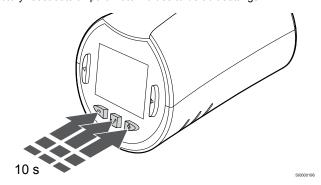
To factory reset the thermostatic head:
