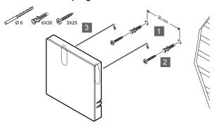
Attach the thermostat to the wall using the screw and wall plug.
