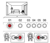
Use buttons < or > to move the pointer (LED flashes red) to the first empty channel needed for the room (no LED). The LED flashed red.
