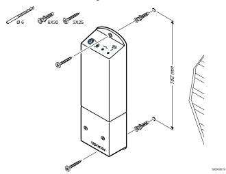
Attach the relay module to the wall using screws and wall plugs.
