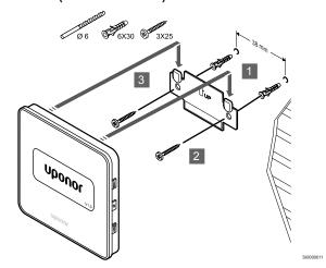
Attach the thermostat to the wall using the wall bracket, screws and wall plugs.
