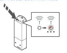
Press and hold the register button on the relay module until the LEDs on the module start flashing slowly.
