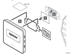
Attach the thermostat to the wall using the wall bracket and adhesive strips
