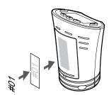
Label the thermostatic heads, where suitable, with the channel numbers they are connected to, for example, #02, #03. For a system with several room controllers, add the ID of each room controller, for example, 1.02, 1.03, 2.02, 2.03.
