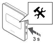
Press and hold the  $\bf OK$  button for about 3 seconds. The settings icon and menu numbers is displayed in the top right corner of the display.
