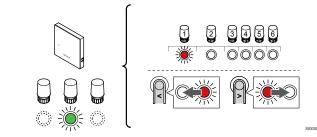
Use buttons < or > to move the pointer (LED flashes red) to a preferred channel.
