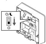
Optional: To activate tamper alarm for the thermostat, set the Disable timer switch to Comfort mode ( $^{\circlearrowright}$ ) before registering the thermostat.
