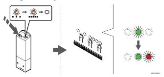
Press and hold the register button on the relay module until the LEDs on the module start flashing slowly.
