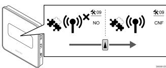
The connection indicator is shown in the thermostat display to show that the registration process begins.
