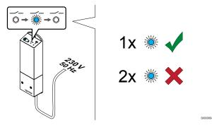
Power up the relay module and count the number of flashes of LED 2 (blue) to ensure it is in normal run mode.
