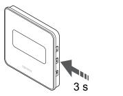
Press and hold the  $\mathbf{OK}$  button for about 3 seconds to exit the settings menu.
