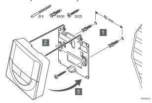
Attach the thermostat to the wall using the wall bracket, screws and wall plugs.
