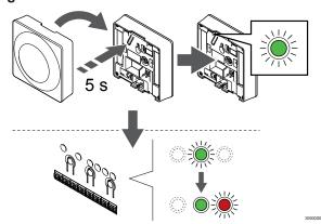
Gently press and hold the registration button on the thermostat, release when the LED starts flashing green (located in the hole above the registration button).
