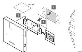
Attach the thermostat to the wall using the wall bracket and adhesive strips.
