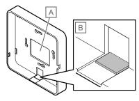
Route cables to the communication module using one of two cable entries.
