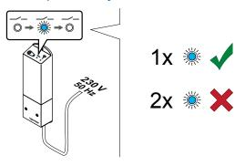
Power up the relay module and count the number of flashes of LED 2 (blue) to ensure it is in normal run mode.
