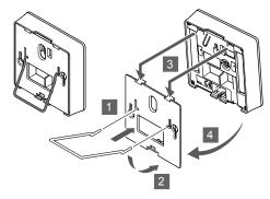
Attach the table stand to the thermostat using the wall bracket.
