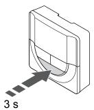
Press and hold the  $\mathbf{OK}$  button for about 3 seconds to exit the settings menu.
