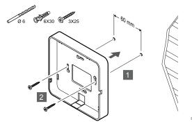
Attach the communication module back mount to the wall using the screws and wall plugs.
