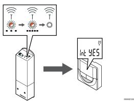
The connection indicator starts flashing in the thermostat display to show that the registration process begins.
