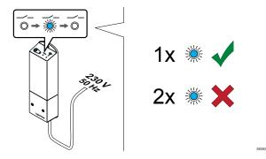
Power up the relay module and count the number of flashes of LED 2 (blue) to ensure it is in two stage additional cooling mode.
