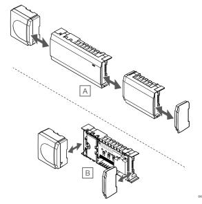
The components can either snap on or off without the need of removing the covers (A, recommended to do on a flat surface or on a DIN-rail), or by sliding them into place when the covers are removed (B).
